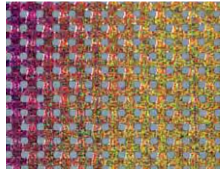
Printed SEFAR® Architecture Vision fabric AL 260/55 and magnified approx. 8 times
