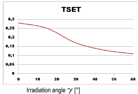
Figure 2: TSET according to DIN EN 410 in the 2-pane make up with low-e coating
